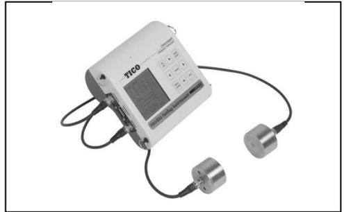
Figure 12. Equipment for ultrasonic on-site tests.
