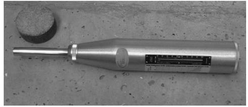
Figure 11. Schlerometer for on-site tests.
