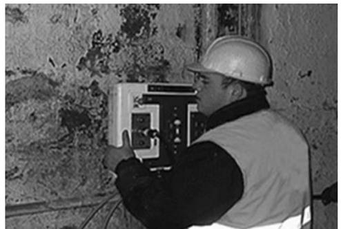
Figure 9. On-site analysis using geo-radar techniques.
