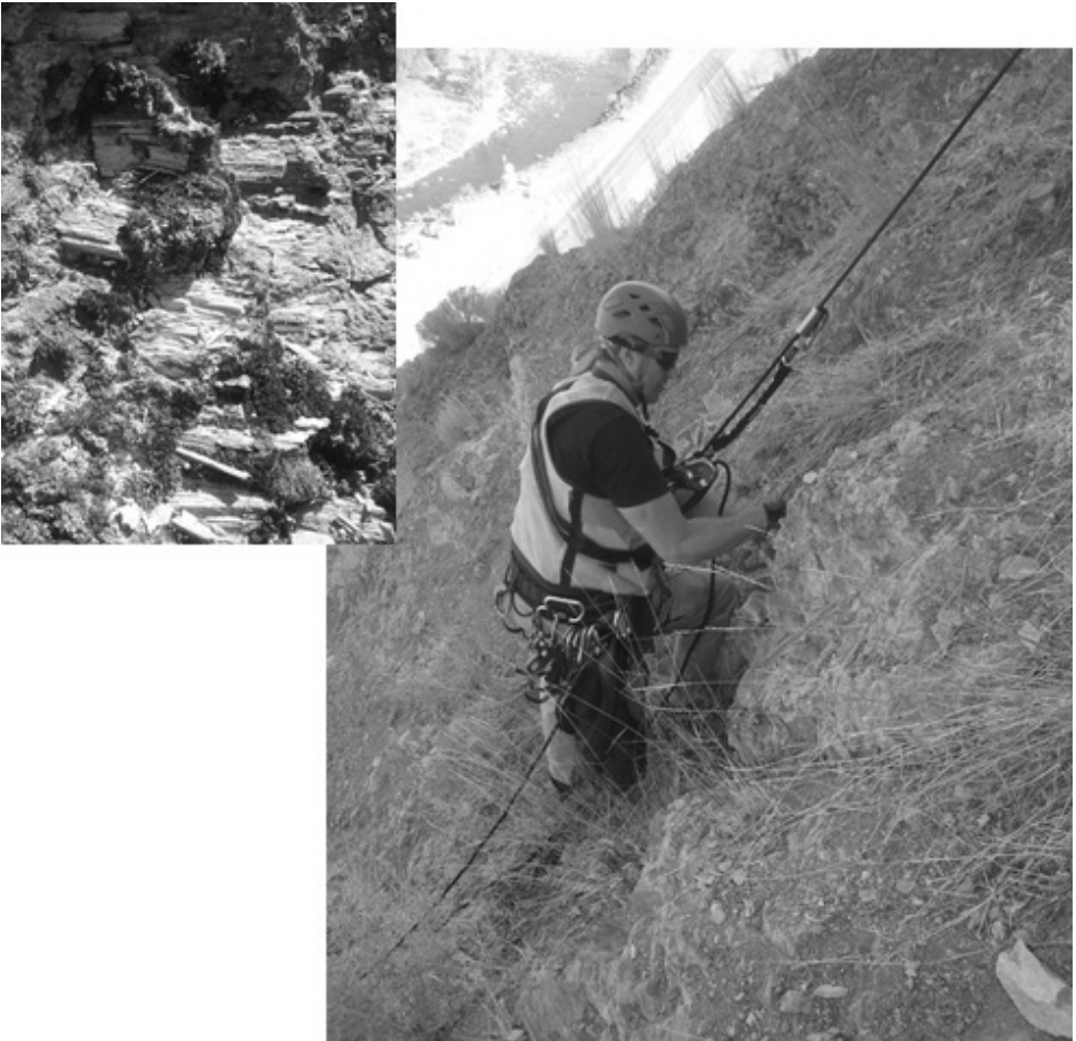
Figure 5. Jim Struthers with MJA using rope access safety techniques sampling for NOA at the contact between the serpentinite rock and the schistose rock units. Photo on the left is a nonregulated fibrous mineral antigorite like the regulated NOA species actinolite and tremolite.
