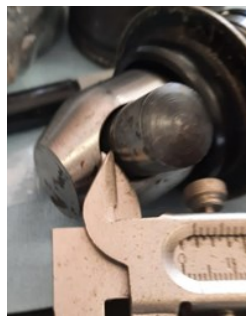
Too much clearance
