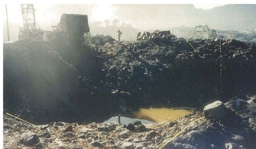
Porgera Mine Explosion - Papua New Guinea – August 2nd, 1994: fire on the bulk truck, around and underneath the bulk emulsion tanks led to the explosion. 11 Fatalities.
