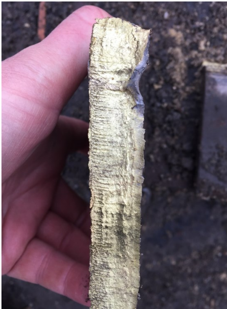
Linear Cutting Charge on Steel Section
